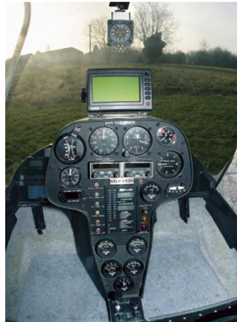
ABOVE Gauges show voltage, oil temperature, oil pressure etc. The tachos show engine and rotor RPM in the Robinson-style (ie crossed needles). The engine is fuel injected, so there is no carb heat gauge.
